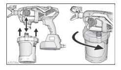
The VacuValve is an important part of your new sprayer. It is used to evacuate the air out of the FlexLiner. Your sprayer will not spray if there is air in the FlexLiner.
