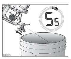
13. If second spray tip was used, remove cleaned spray tip from spray tip guard and install second spray tip. See Spray Tip Installation, page 23. Repeat steps 11 and 12 to clean second spray tip.
