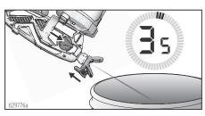
**IMPORTANT!** For best results, do not spray more than one cup of water through the tip while cleaning. If more flushing is needed, remove the tip from the sprayer to avoid excessive wear.
