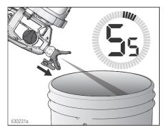
Reverse the spray tip to UNCLOG position, pull the trigger for five seconds. Release the trigger.
