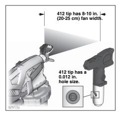
First digit when doubled = approximate fan width. Last two digits = tip hole size in thousands of an inch. For an 8 to 10 in. (203 to 254 mm) fan width and 0.010 (0.25 mm) hole size, order Part No. ...410.
