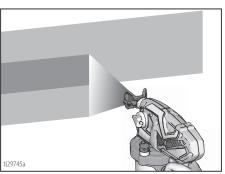
Rotating the spray tip guard changes the pattern to either the vertical or horizontal orientations.
