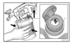
Stop squeezing the FlexLiner and snap the VacuValve cap closed. You will hear the cap click when it is closed properly.
