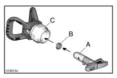
Insert Spray Tip. Spray tip must be pushed all the way into the tip guard.
