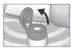
5. Open VacuValve cap. Tilt the sprayer so the VacuValve is the highest point, causing any air in the FlexLiner to rise to the VacuValve. Gently squeeze the FlexLiner to evacuate all air through the VacuValve air hole. Once you see material enter the VacuValve reservoir, all air should be evacuated from the FlexLiner.
