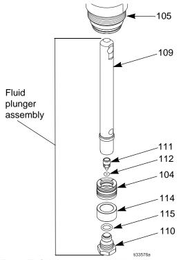
Fig. 6 Fluid plunger assembly
