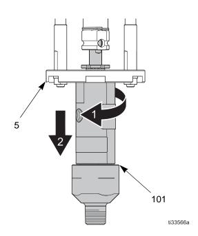
Fig. 4 Remove fluid cylinder
