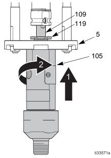
Fig. 11 Reconnect fluid cylinder
