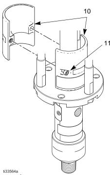
Fig. 2 Remove dust cover
