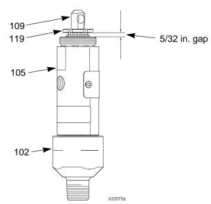
Fig. 9: Tightening the packing nut
