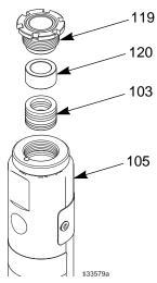
Fig. 8 Top packing seal assembly
