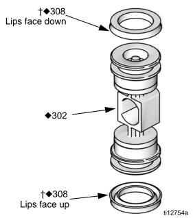
Fig. 16. Pneumatic Valve U-cup Installation
