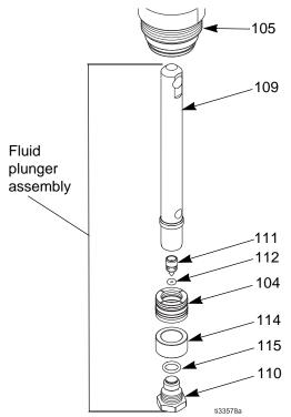
Fig. 10 Fluid plunger assembly
