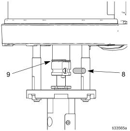
Fig. 3 Retaining spring and connector pin
