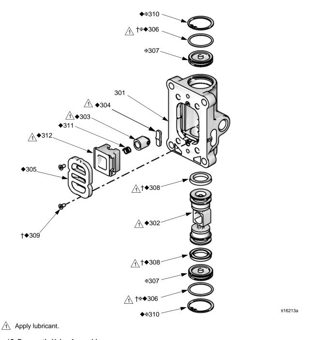
Fig. 15. Pneumatic Valve Assembly
