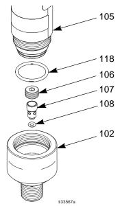
Fig. 5 Fluid cylinder cap assembly
