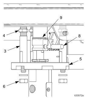
Fig. 18 Retaining spring and connector pin
