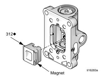
Fig. 17. Pneumatic Valve Cup Installation
