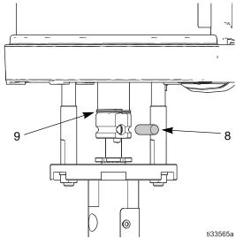
Fig. 12 Retaining spring and connector pin
