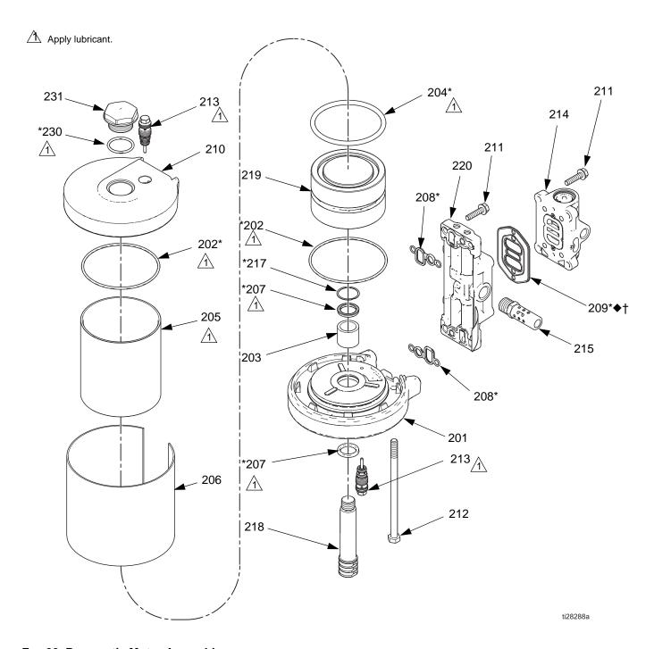
Fig. 20. Pneumatic Motor Assembly
