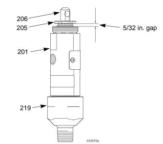
Fig. 10: Tightening the packing nut
