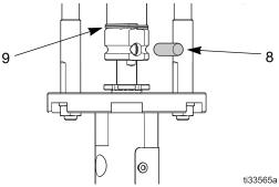
Fig. 4 Retaining spring and connector pin
