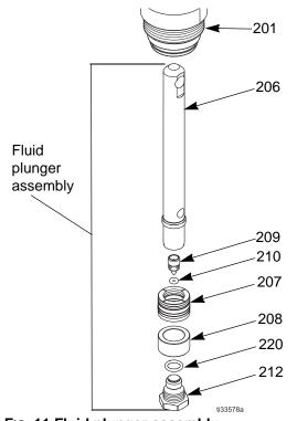
Fig. 11 Fluid plunger assembly
