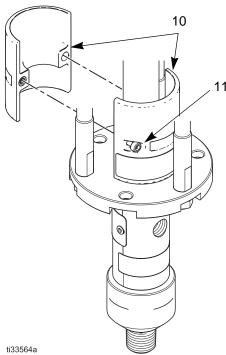
Fig. 3 Remove dust cover
