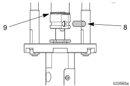
Fig. 13 Retaining spring and connector pin
