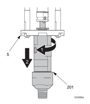
Fig. 5 Remove fluid cylinder
