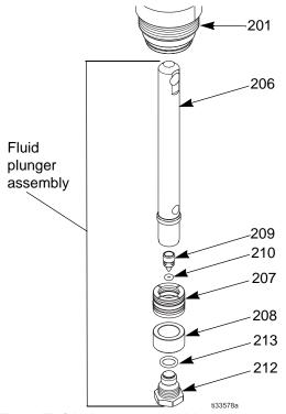
Fig. 7 Fluid plunger assembly
