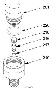
Fig. 6 Fluid cylinder cap assembly
