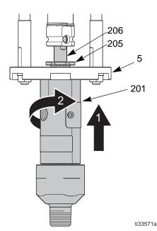
Fig. 12 Reconnect fluid cylinder
