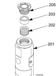
Fig. 9 Top packing seal assembly
