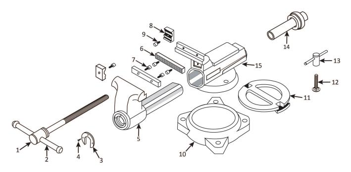
Figure 1. Vice Exploded Parts View
