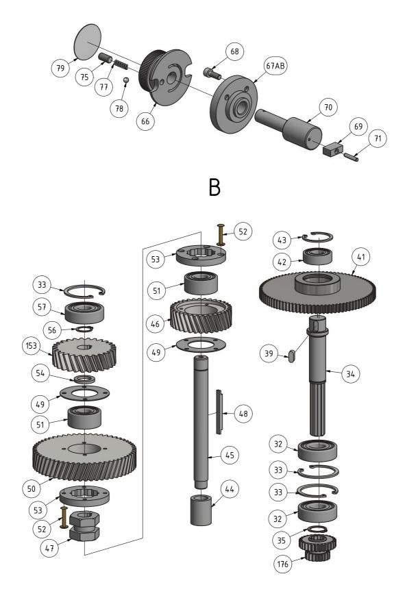
8-3: Bohrkopf - Drilling head
