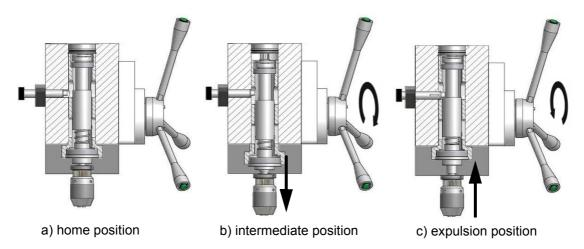
Img.4-18: Functional diagram of the drill drift (sectional view)
