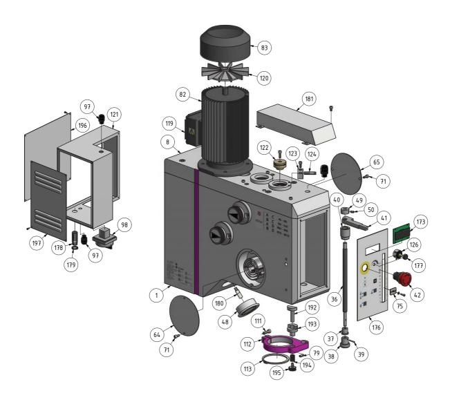
7-8: Bohrkopf - Drilling head
