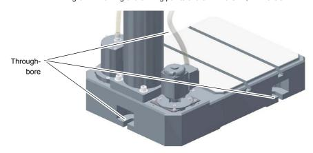
Img.3-2: Marking of the fixing points of the DH 32 GSV
