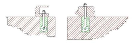
Img.3-3: Example for the floor fixture DH 28 GSV and DH 32 GSV
