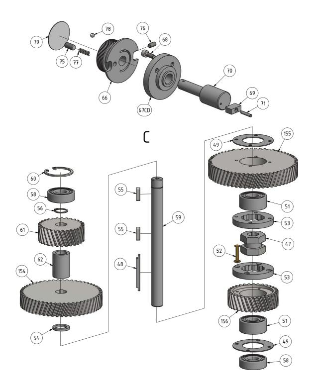
8-4: Bohrkopf - Drilling head
