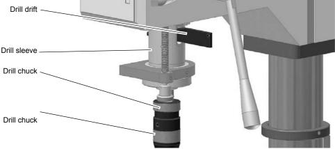
Img.4-7: Disassembly with drill drift
