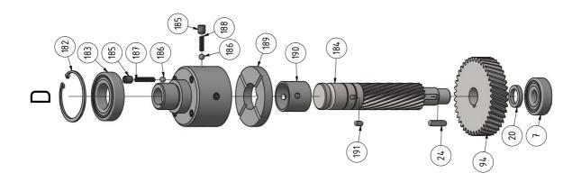
7-6: Bohrkopf - Drilling head
