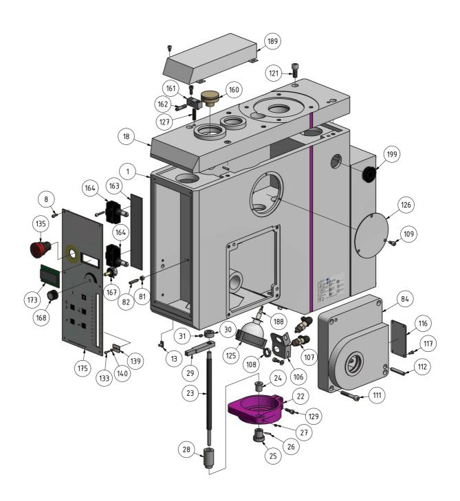
8-8: Bohrkopf - Drilling head
