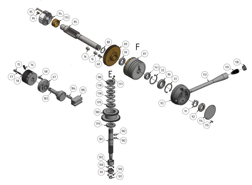
8-7: Bohrkopf - Drilling head
