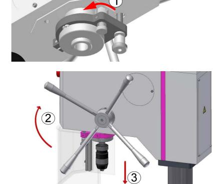
Img.4-8: Disassembly with integrated drill drift
