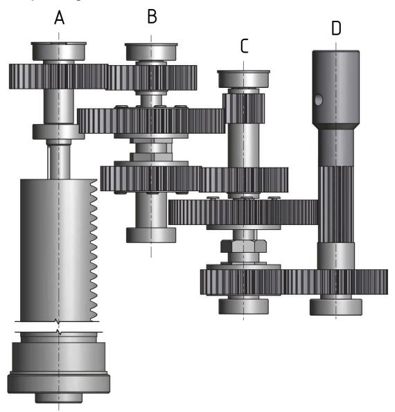
8-1: Bohrkopf - Drilling head
