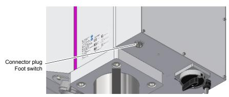
Img.3-6: Connector plug foot switch
