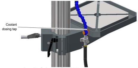
Img.4-21: Coolant shut-off tap and doser
