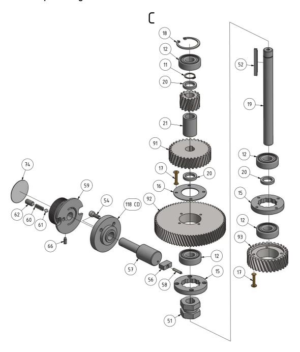
7-4: Bohrkopf - Drilling head
