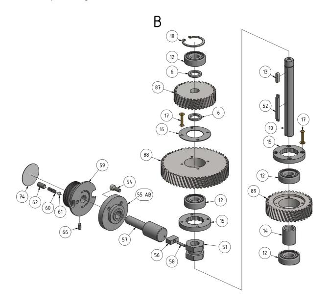
7-3: Bohrkopf - Drilling head
