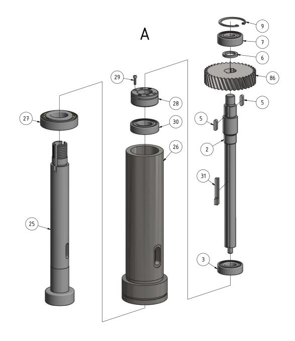
7-2: Bohrkopf - Drilling head
