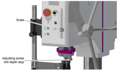
Img.4-3: Drill depth stop
