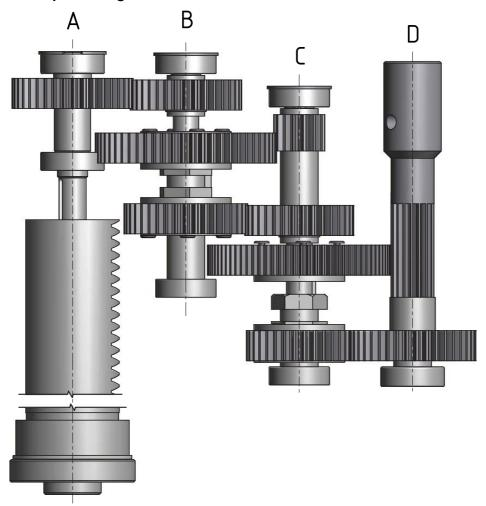
7-1: Bohrkopf - Drilling head
