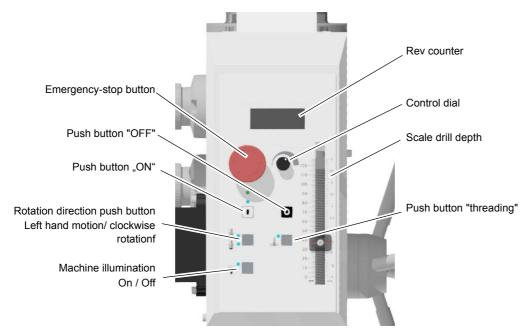
Img.4-2: Operating elements on the control panel
