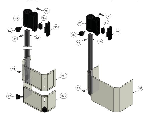
7-9: Bohrfutterschutz- Drilling chuck protection
