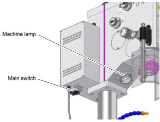
Img.4-11: Machine lamp
