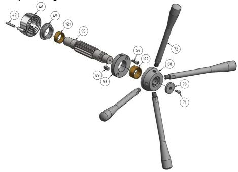
7-7: Bohrkopf - Drilling head
