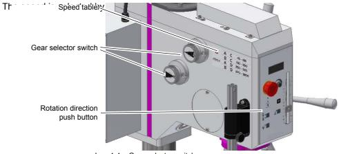
Img.4-4: Gear selector switch
