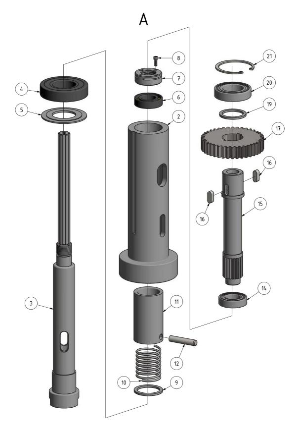
8-2: Bohrkopf - Drilling head
