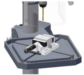
Img.4-1: seats for slot nuts
