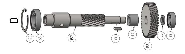
8-5: Bohrkopf - Drilling head
