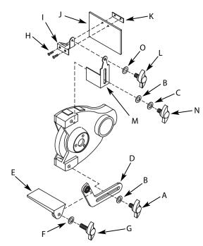
Figure 1 – Left Tool Rest and Eyeshield Assembly
