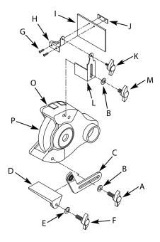
Figure 1 - Left Tool Rest and Eyeshield Assembly
