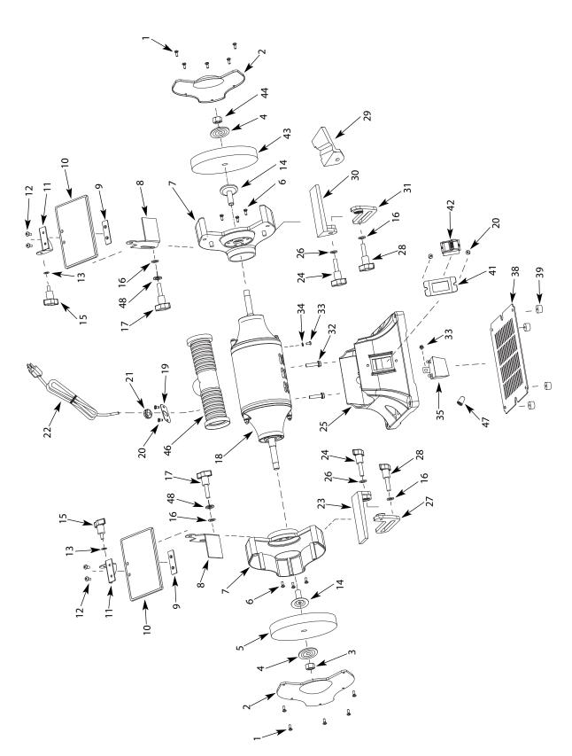
Figure 5 – Repair Parts Illustration for 9682072A, 6" Bench Grinder
