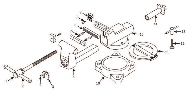
Figure 1. Vice Exploded Parts View
