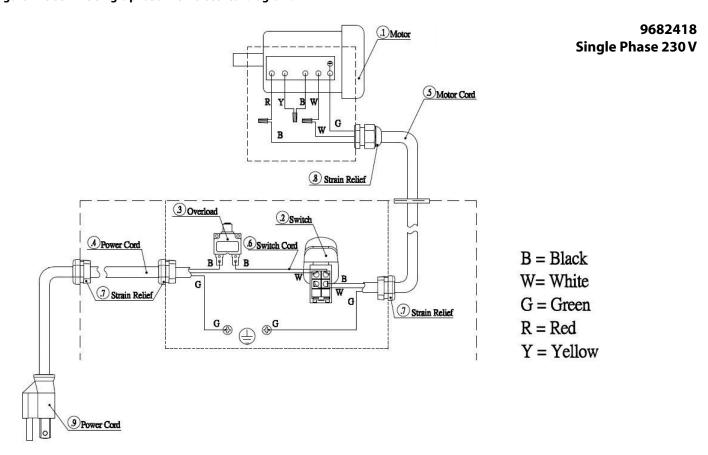
Figure 8 - 9682418 single phase 230V electrical diagram.
