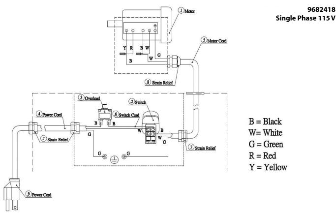
Figure 7 - 9682418 single phase 115V electrical diagram.
