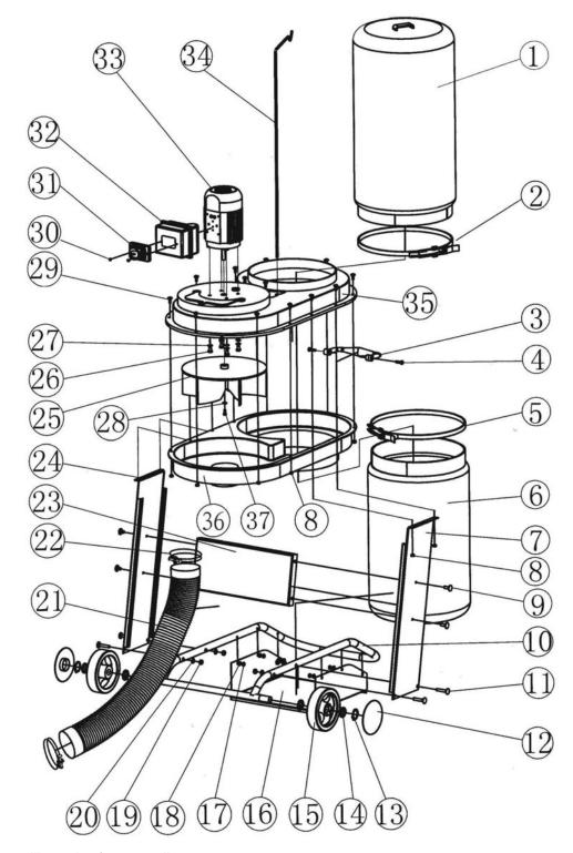
Figure 3 – Repair parts illustration for Dust Collector.
