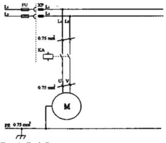
Figure 2 - Circuit diagram.
