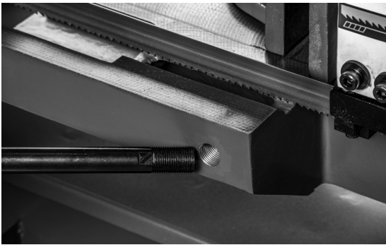
Match long rod's screw to hole just below vise.
