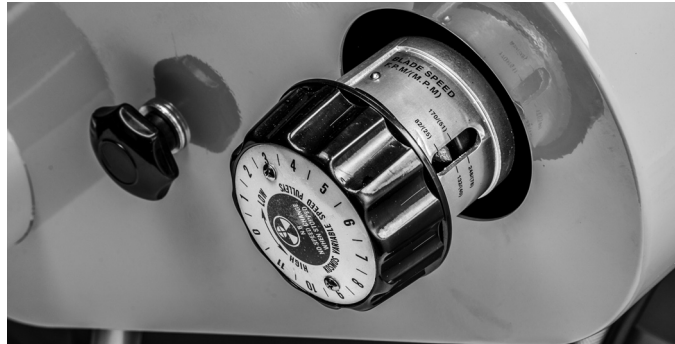
Figure 13 – Blade speed selector.
