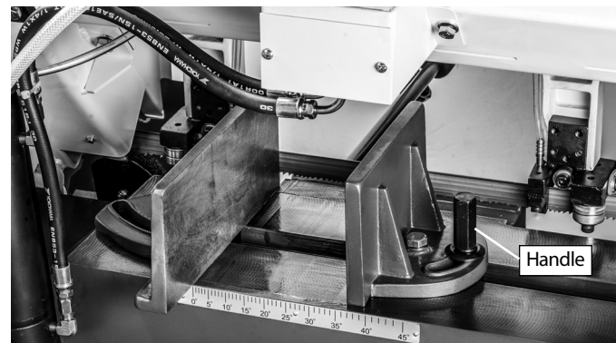
Figure 11 - Adjust angle of vise.
