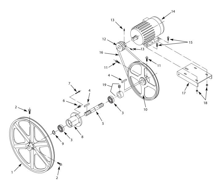
Figure 13 – Repair parts illustration for motor and lower wheel.
