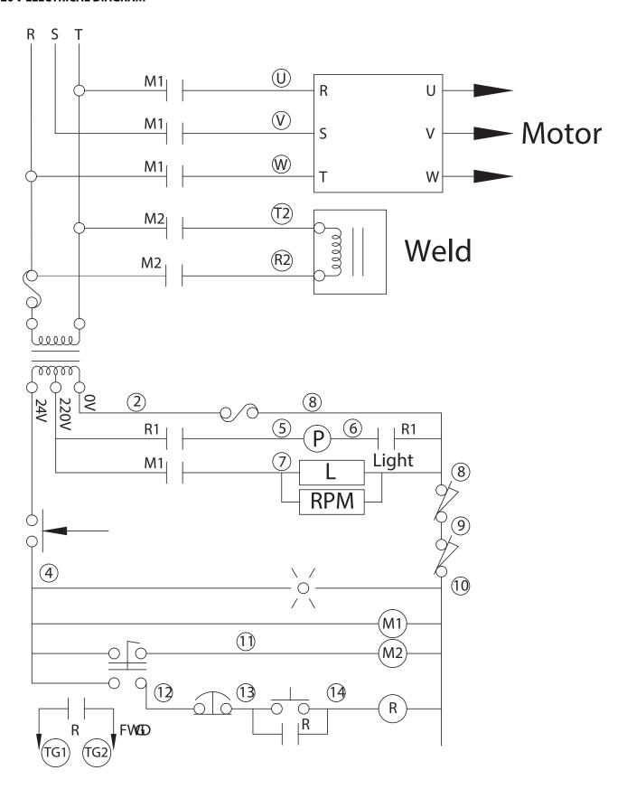
Figure 9 – 9683120 electrical diagram, 220 V.
