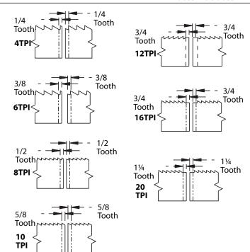
Figure 7 – Tooth spacing (TPI = teeth per inch).
