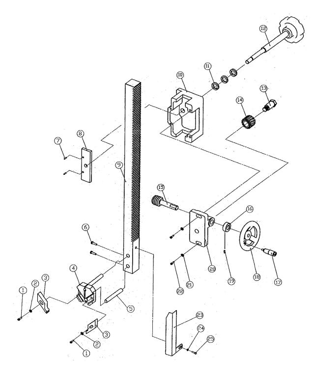
Figure 15 – Repair parts illustration for guide post.
