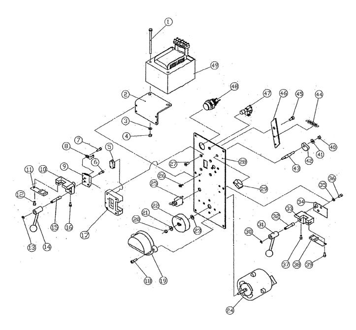
Figure 16 - Repair parts illustration for welding station.
