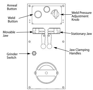
Figure 4 – Blade welder controls.
