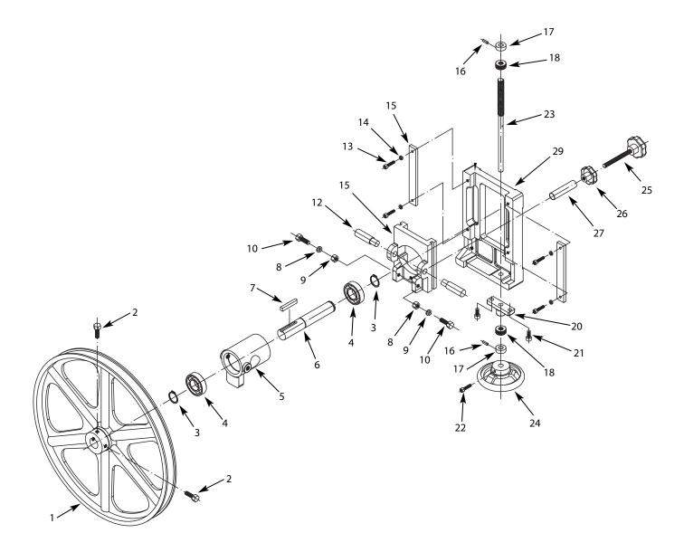
Figure 14 - Repair parts illustration for upper wheel.
