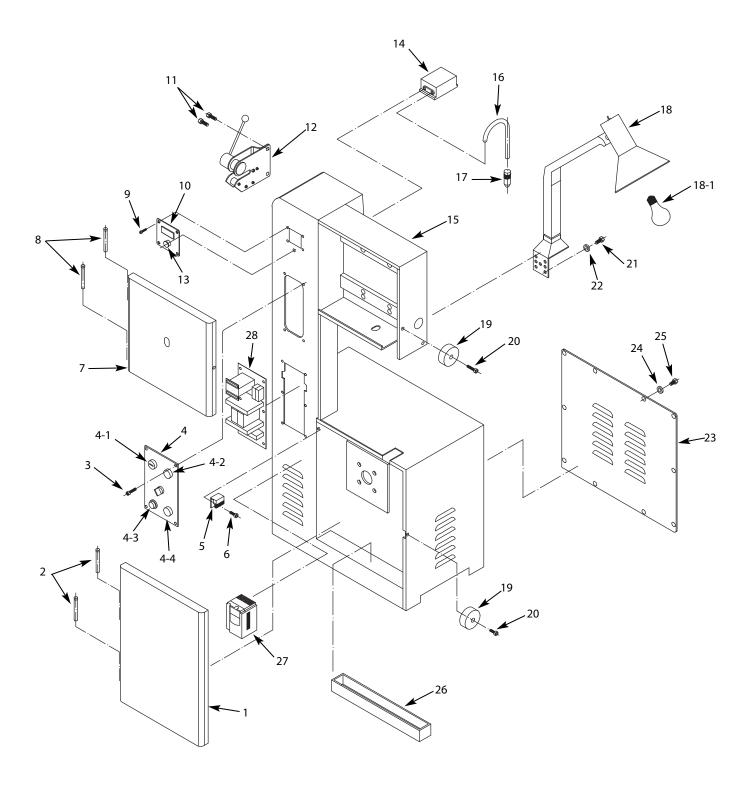
Figure 11 – Repair parts illustration for cabinet.
