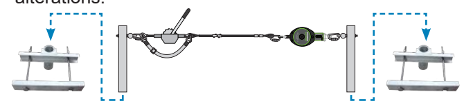
Fig. G. FormLink (FS-EX2502) 3 different applications: Clamped around rebar or a finished column, or mounted on a finished wall (See p. 8-9).
