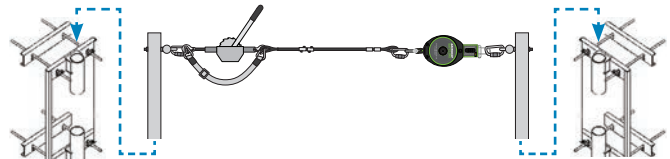
Fig. F. EZLink Double Connector (FS-EX2502-DBL) Attached directly to the column rebar cage—six (6) # 9 rebar or larger—without the need for decking alterations.
