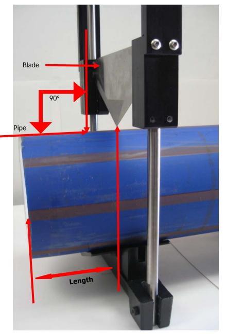
Make sure pipe is properly placed in V-Base. Blade must be perpendicular to the pipe before a cut can begin.
